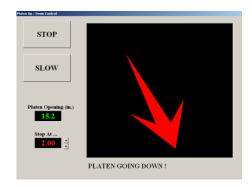
LOAD APPLIED SAFETY FEATURE. Should anything come in contact with the bottom platen while the machine is traveling down at fast speed, the Compression Tester's "load cell" senses it and this safety feature stops the machine, preventing damage or erroneous test results.
